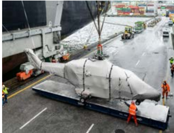
Helicopter shipped from La Spezia to Nhava Sheva with one lifting point: the rotor.
